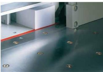
AIR TABLE The front and rear table of the IDEAL 7228-06 LT are equipped with air jets for easy and effortless handling of large paper stacks.
