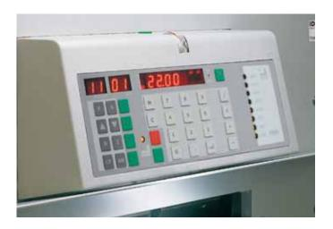
**ELECTRONIC CONTROL MODULE** Professional, programmable control module for the power backgauge (99 programs with 99 steps in each program).
