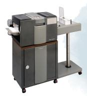
The Posmate 6 offers the advanced heavy duty Desktop Pressure Sealer. It provides the Superior FRR (Friction Reverse Roller) with a cooling system. Up to 1,400 Sheets can be loaded in the feeder and processed at speeds up to 9,000 sheets per hour. It also provides great sealing quality with the 4 Press rollers.
